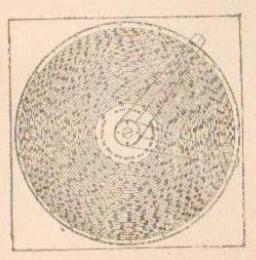
Will solve any problem in multiplication, division and proportion as quickly as the ordinary ten-inch straight slide rule and it will give the result with a maximum probable error of 1 in 30,000. This instrument has two Logarithmic Scales, one 30 inches long and the other, a spiral, 75 feet long. Two results to every problem can be read. The result given by the short scale can be read to three figures and the result on the 75 foot scale can be read to five figures as 98,687.
