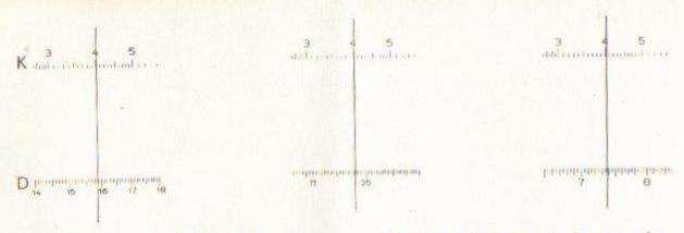
To find the cube root of a number greater than 1 000 write it down as the product of a number between 1 and 1 000 and a power of 10 so that the power is divisible by 3, ie  $4000 = 4 \times 10^3$
