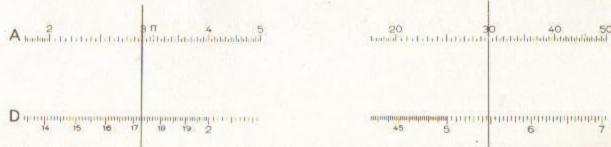
To find the square root of a number greater than 100 write it down as the product of a number between 1 and 100 and an even power of 10, ie  $300 = 3 \times 10^2$  (see over for example)
