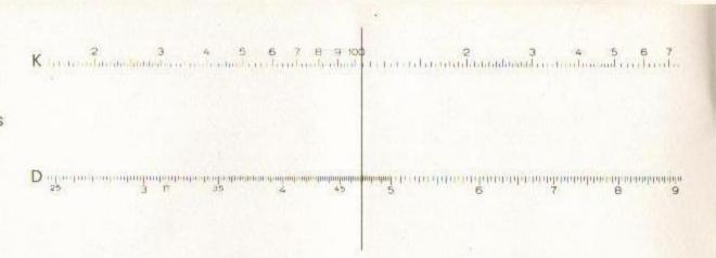
For finding cube roots we project from the K scale on to the D scale. Care must be exercised in selecting the relevant part of the K scale; eg  $\sqrt[3]{4}$ ,  $\sqrt[3]{40}$ , <sup>3</sup> √400 each have different significant figures in their answers. The following illustrations show the settings for each of these cube roots using each of the three parts of the K scale
