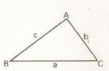
Example: Given a = 24.3, b = 16.5, A = 65° Set cursor to  $S_{65}$ Set  $C_{243}$  to cursor Set cursor to  $C_{165}$  and read on S scale 38° (the value of B) Then  $C = 180^{\circ} - (65^{\circ} + 38^{\circ}) = 77^{\circ}$ Set cursor to  $S_{77}$  and read on C scale 261 (ie 26.1) and the triangle is solved
