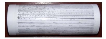
The second prototype is shown above. The scale I have drawn is shown below. The scale consists of two identical scales side by side drawn in the style of a Gridiron. Each scale consists of four decades of logarithms covering the cotangents from 0 degrees 55 minutes and 89 degrees 15 minutes. A cosine scale produced with two decades of logarithms occupies the bottom left quadrant.
