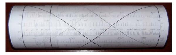
This second design works very well. The accuracy is limited by the accuracy of my drawing and the length of the log curve. By adding a vernier scale to the minor cursor I can however get an extra significant figure when reading the answer.
