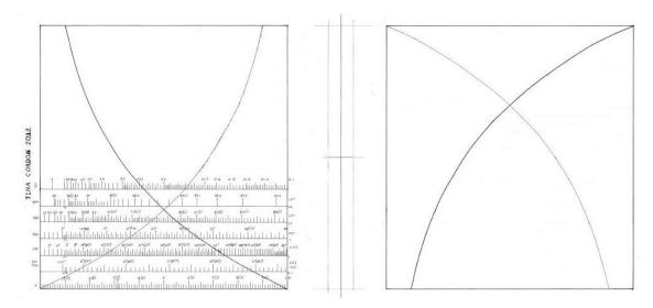
The drawing to the left in the above image shows the design for the base scale. The drawing to the right shows the design for the major cursor.
