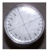
For example 6 is on the third log section about  $1/8^{th}$  of a rotation along that section. 7 is also on the third section about  $3/8^{th}$  of a rotation along. Using the dial 3 + 3 = 2 according to the rules of clock arithmetic and  $1/8^{th} + 3/8^{th} = \frac{1}{2}$ , therefore the answer will be found about half way along the section labelled 2 where 4.2 is indeed found.
